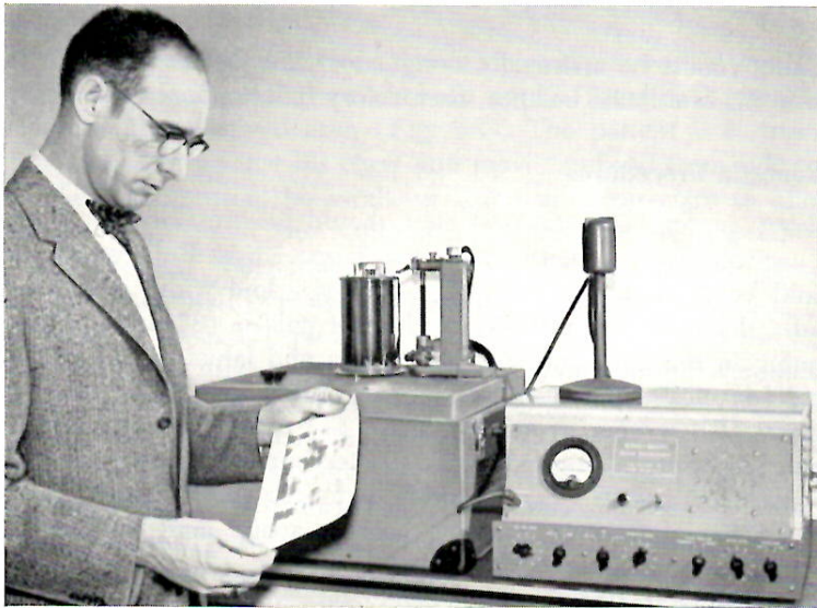
Fig. 4. Visible speech is analyzed by the Sound Spectrograph, which charts the speech pattern, frequency vs. time, related to intensity. Each vowel and consonant display can be compared to normal, thus showing the weakness of the patient's pattern of speech.
